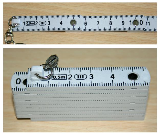
Figure 1 Example of the 0.5 m x 13 mm folding ruler
